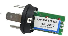
upper part of a connector (Hirschmann type GSP). Its design makes it ideal for mounting in tubular housings. The plug is widely used in industry. With this arrangement, customer-specific probes with integrated transducers can be realized at low cost. To increase vibration resistance, the Type 406 can also be supplied encapsulated. Delivery without connector is also possible.
